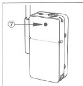
Potentiometer for adjustment of attenuation
